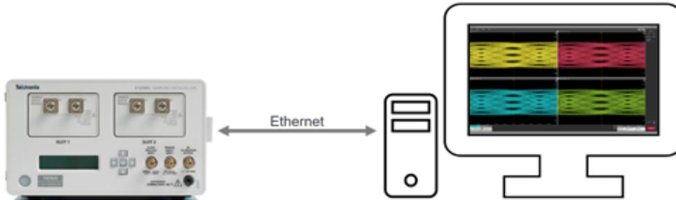
1. Connect the CAT6 Ethernet cable to the LAN connector on the rear panel of the instrument.
