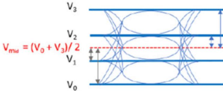
$V_{mid}$  is computed as average of  $V_0$  and  $V_3$ .
