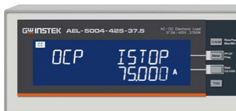
Turbo ON, OCP Istep 7.5 A Istop 75A 测试结果画面
